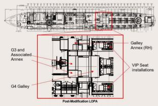
The concern with relocating the galley complex to a location where it had never been situated before was whether the floor and monocoque fuselage had the necessary static strength to support the weight of the monuments during worst case flight gust conditions.
