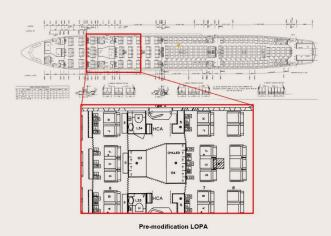
The pre-modification passenger arrangement is shown above and the post-modification VIP lay-out is shown to the upper right.
