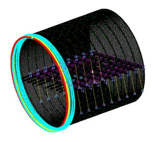
This model was used to compare the impact of MAX PAX (maximum passenger occupancy) seat loading with the loading introduced by the Galley Complex.
